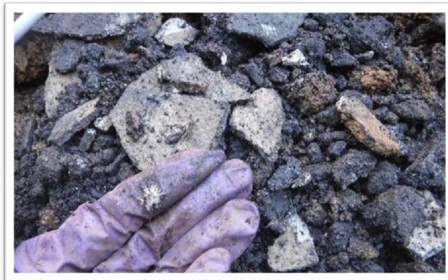
A sample showing asbestos waste.
